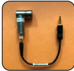
TEST MIC,ASM 46AO-S3,DSA7K connected with a mic cable (mic cable CAB-MP35-174-17CM is coming together with the DSA7000 analyzer)
