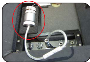
FOAM, LUX RHI p/n 20878000 support for test rec & coupler
