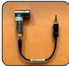
TEST MIC,ASM,46AO-S3,DSA7K connected to a mic cable (mic cable CAB-MP35-174-17CM, delivered together with the DSA7000/ APX511 analyzer)
